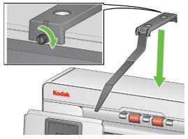
NOTE: To change the dangler remove the mount, unclip the dangler, and snap the desired dangler into the slots as shown.
