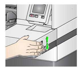
• Press the lower portion of the button on the side of the scanner to lower the workspace table.
