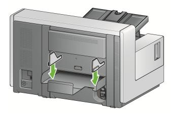
NOTE: The locking knob on the bottom of the exit tray can be loosened to allow you to slide the tray forward or backward to accommodate the size of the documents you are scanning.
