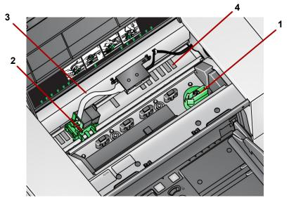
1 Feed module release knob — turn this knob to release the feed module from it's position for cleaning or replacement. Turn the arrow to right to disengage the feed module.
