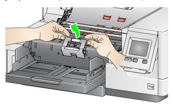
5. Manually rotate and wipe the separation roller tires with a roller cleaning pad. For best results wipe parallel to the ribs in order to remove any residue between the ribs.
