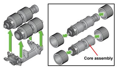
8. Install each new tire by gently pulling it over the core assembly. The tires do not need to be installed in any specific orientation.
