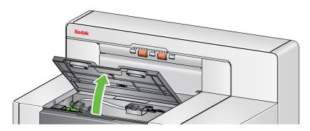
NOTE: If you do not want to remove the output tray, you can lift the front of the output tray, then lift the printer access cover and position the printer access cover behind the height adjustment tab.
