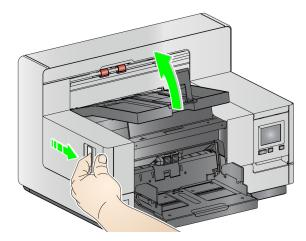
3. When finished cleaning the scanner or replacing a consumable, close the scanner cover with both hands.
