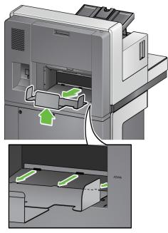
The scanner comes with 3 different-sized, magnetized danglers, which can easily be changed based on the document set you are scanning.
