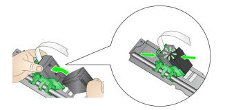
4. Rotate the printer carrier back and snap it in place.
