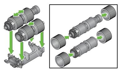
10. Press the upper and lower housings together until they snap into place.
