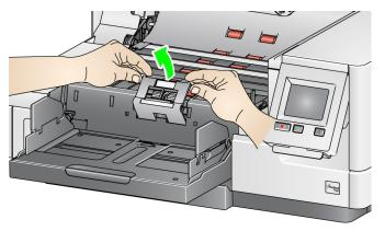
NOTE: The separation roller cover is spring-loaded. Hold the separation roller cover back until you remove the separation roller, then gently lower the separation roller cover back in place.
