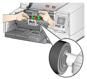
4. Gently release the separation roller cover back in place and close the scanner cover.
