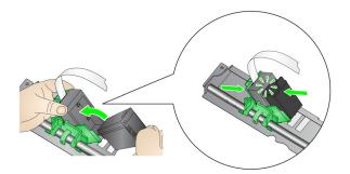
5. Rotate the printer carrier and snap it in place.
