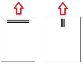
To enable feeding in any direction it is common that patch pages are created with patch patterns on each edge of the page.
