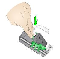
3. Snap the ink cartridge into the printer carrier as shown.
