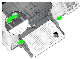
Adjusting the height of the input elevator — the input elevator can be set to accommodate stacks of 25 or less, 100, 250, 500 or 750 documents of 20 lb./80 g/m<sup>2</sup> bond paper. Input elevator settings are made through your scanning application software (i.e. TWAIN Datasource, ISIS Driver, or VRS).
